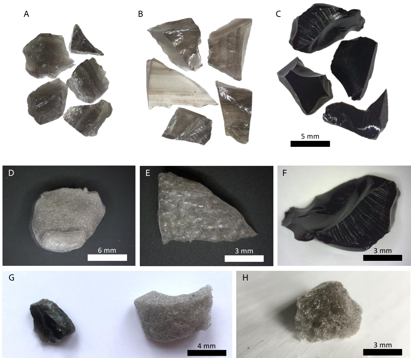
Figure 4: Photographs of obsidian chips before and after heating in the microwave kiln. Before heating, we used obsidian chips from [A] Mono Craters (U.S.A.), [B] Arteni (Armenia), and [C] Hrafninnuhryggur (Iceland). Examples of these chips after heating appear in panels [D], [E], and [F]; note that the Hrafninnuhryggur obsidian in [F] did not foam up because at 700 W for 15 minutes, the temperature and time were insufficient to promote bubble growth for the low H_2O concentration in this obsidian. In [G] and [H] we show an example of the Hrafninnuhryggur obsidian that was held for longer (20 minutes) before and after, where [H] is the same pumice product as in [G] but seen from a different angle. The scale bar in [C] applies to [A] and [B].
